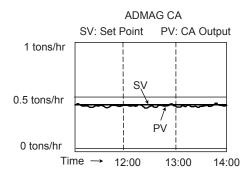
The ADMAG CA output is stable without large output fluctuations
