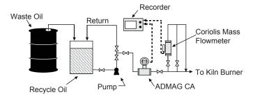
The ADMAG CA was tested in series with the Coriolis meter. The test conditions were as follows:
