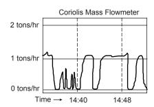
The suspected cause for the output fluctuation is the variation in the fluid's density
